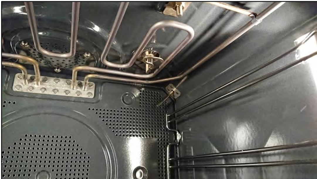
Fig. 4: One of the two antennas in the cavity (© Miele)
